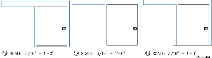
Single Horizontal Manual Slide Door with Backup Casings and Cap Channels
